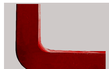
20% thicker at bend & heel
